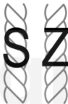
Fig.7.16: ‘S’ Twist and ‘Z’ Twist
